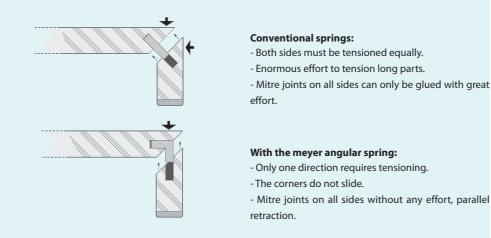
Easy preparation without special machines! A table cutter and notching blades are sufficient. As no springs can jam, a safe and quick gluing process in frame presses is possible. meyer angular springs are available in different sizes and angles. Need a different angle bracket? Ask us!
